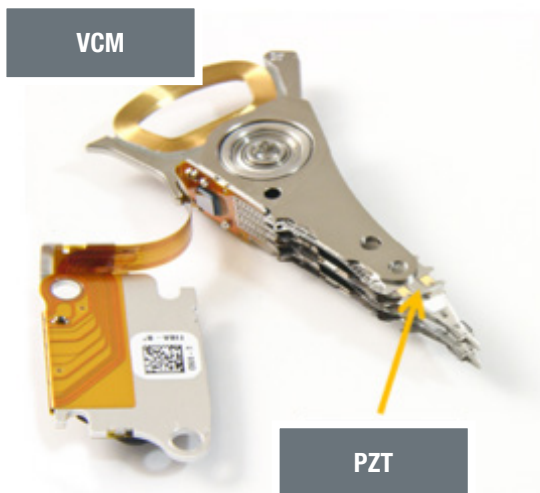
Figure 4. VCM and PZT loops work together
