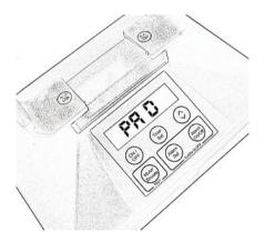
Note: Deafgard will display error messages on the LCD if a fault occurs. If this happens perform a reset on the unit by removing and re-inserting of all batteries. If error remains contact the Technical Advice line. The following are the most frequently asked questions regarding the Deafgard unit, with a quick checklist to follow:
