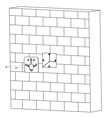
Figure 3-2 Secure Base Plate
