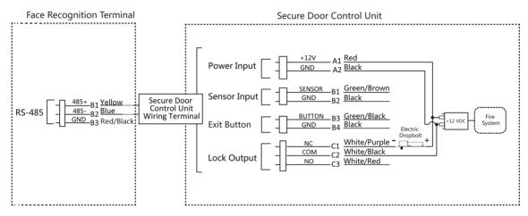
**Figure 4-4 Wire Secure Door Control Unit**
