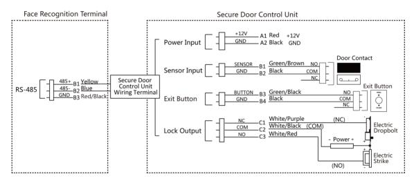
Figure 4-2 Secure Door Control Unit Wiring
