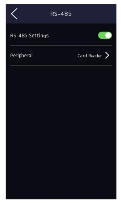
Figure 7-7 Set RS-485 Parameters
