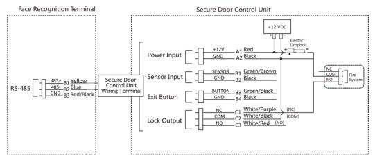
**Figure 4-6 Wiring Secure Door Control Unit**
