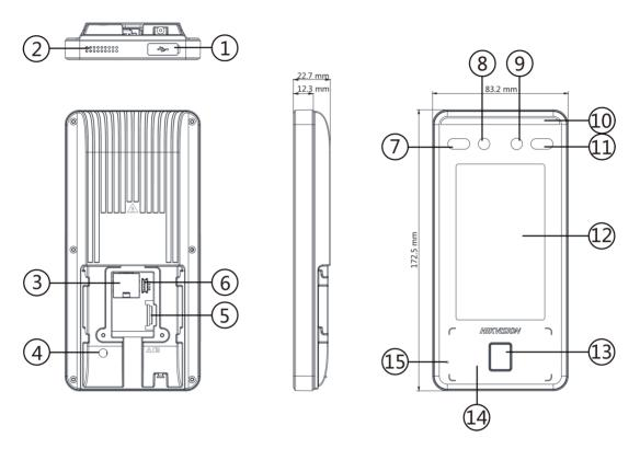
**Figure 2-1 Face Recognition Terminal Diagram**
