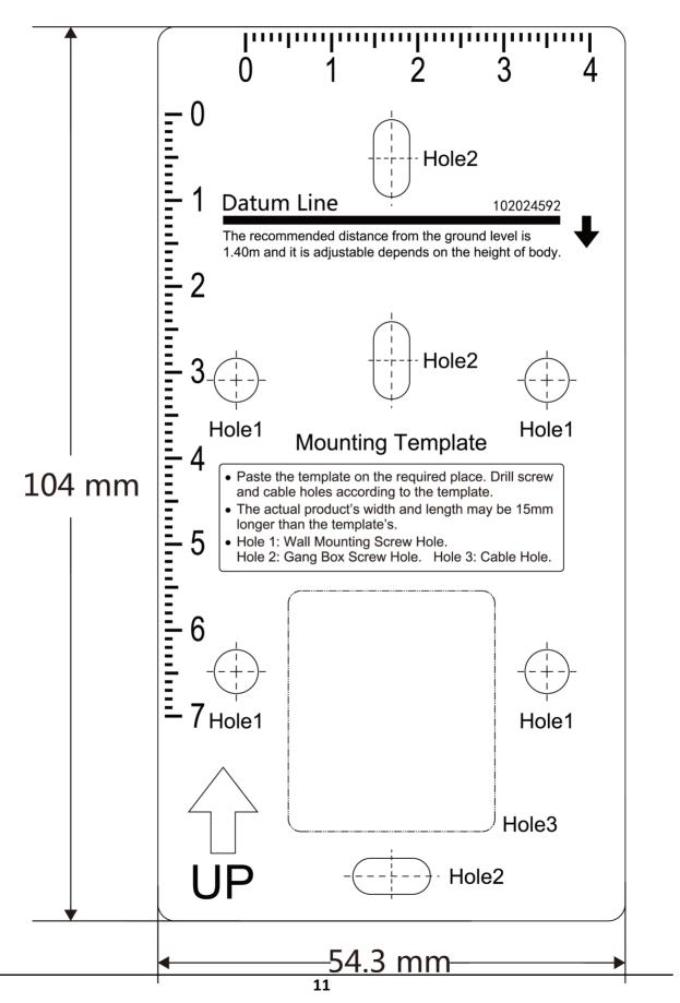
**Figure 3-7 Mounting Template**
