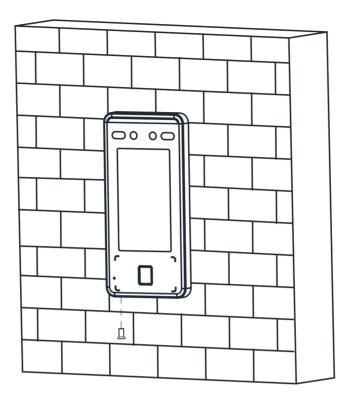
Figure 3-10 Secure Device
