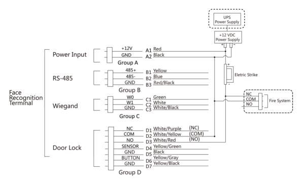
Figure 4-7 Device Wiring
