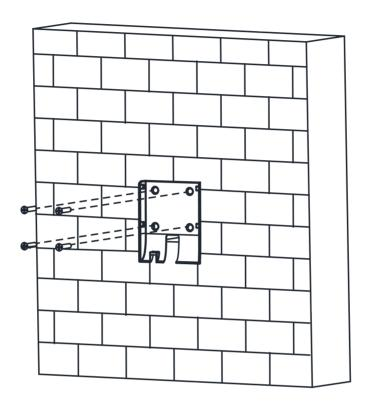
Figure 3-8 Install Mounting Plate
