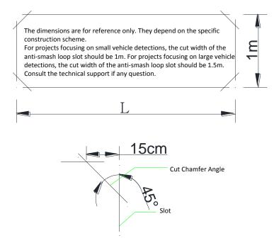
Figure 2-1 Slot Cutting Detail Drawing
