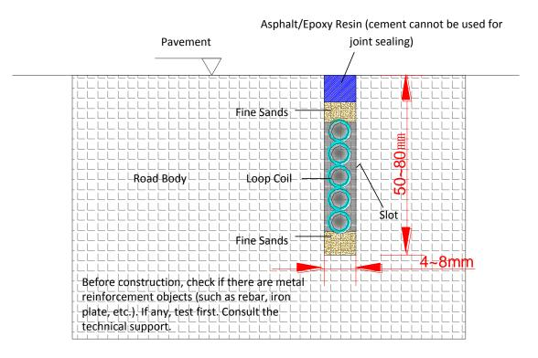
Figure 2-2 Sectional View of Loop Construction
