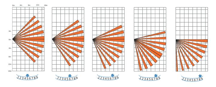
There are 5 scales in the vertical direction to adjust the detection distance. The default angle is A and the detection range is 15 m.
