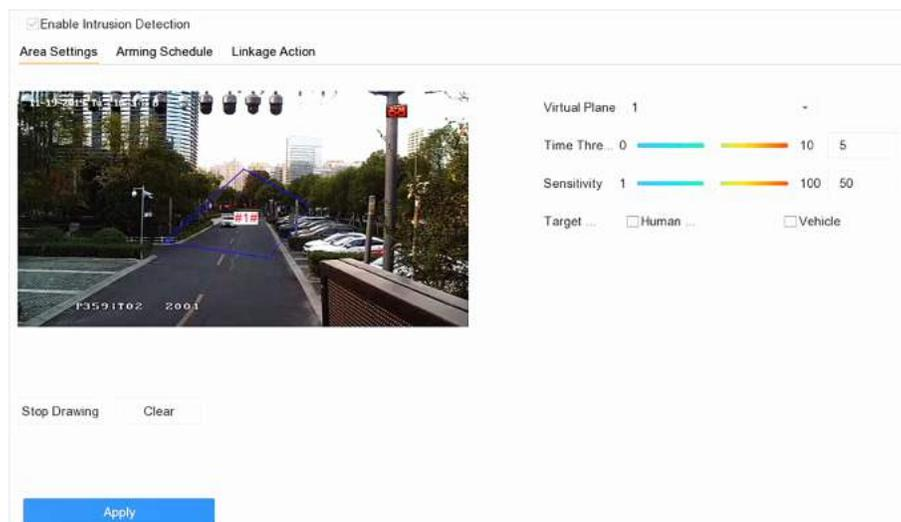
**Figure 6-6 Intrusion Detection**
