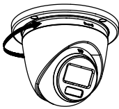
Figure 2-19 Snap Camera into Installation Plate
