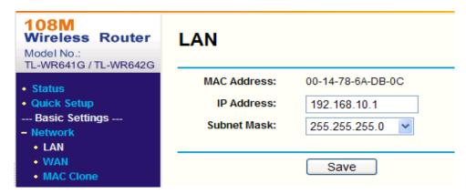
Figure A.2.2 Set the LAN parameters
